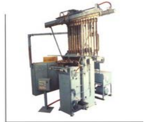
Pull-Down Broaching Machine with Auto Tool & Fixture Changers
